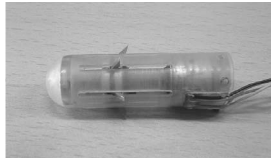
Fig. 4 Fabricated legged microrobot
